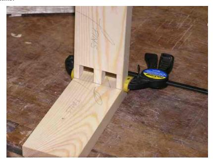
Using a sharp scriber or bradawl, mark the position of the tails. Be careful not to move the pin piece while doing this. You may darken the scribed lines with a pencil for visibility.
