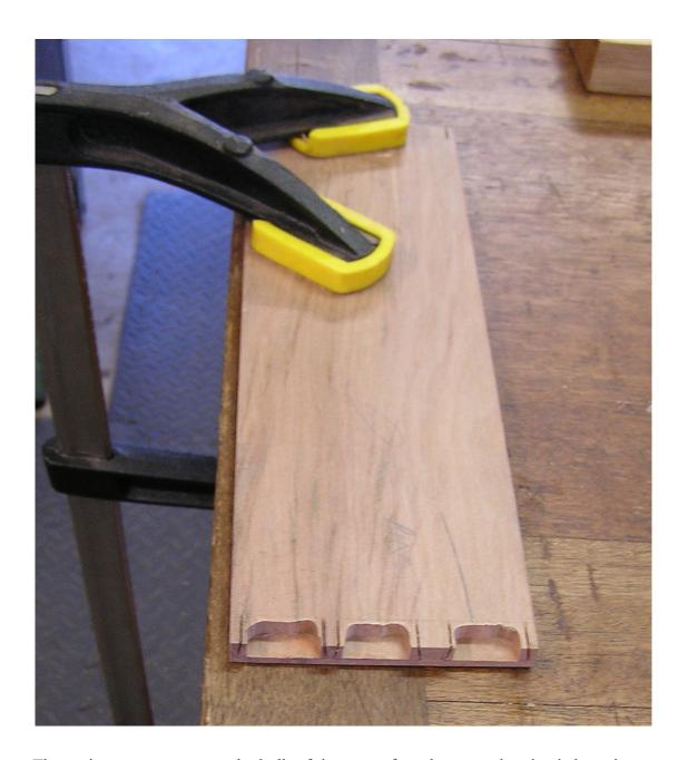
The easiest way to remove the bulk of the waste from between the pins is by using a router. Set a small cutter to the depth of the pins and carefully remove the waste. Do not route right up to the lines, and be sure the router cuts no deeper than the marked line.
