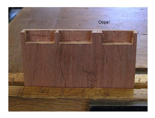
With the side flat on the bench, pare down to the gauged line.
