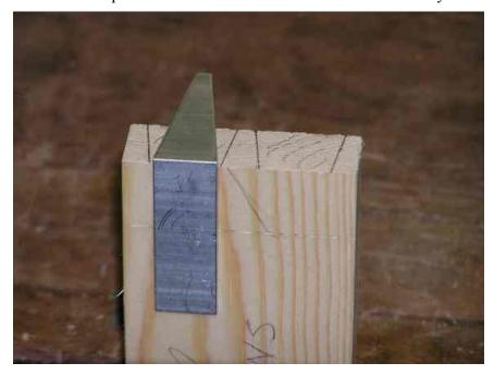
Using a try square held against the end of the wood, mark the pins on the inside and outside faces, and again, mark the waste.
