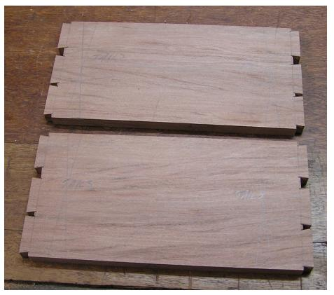
Clean up the tails carefully, and test fit them. Do not force the joints together. They should go together with no gaps, and be a firm but not force fit. To separate the joints after testing, place the tail piece on the bench with the pin piece vertical. Hold the pin piece firmly with the tails slightly above the bench, and strike the tail piece firmly with your hand or a soft-faced mallet. Do not try to wiggle the joints apart.
