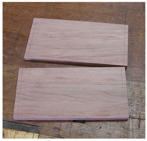
Hold the pin piece in position against the tail piece, and carefully mark the location of the tails using a scratch awl.
