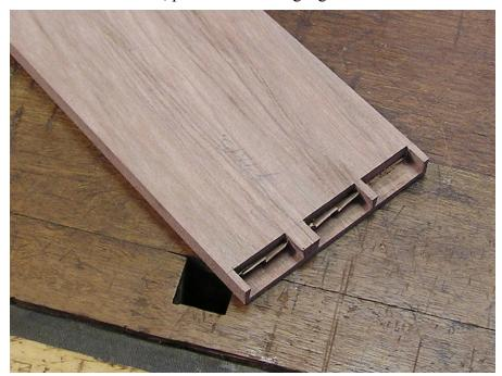
Clean out the sockets and, if necessary, straighten the pins.
