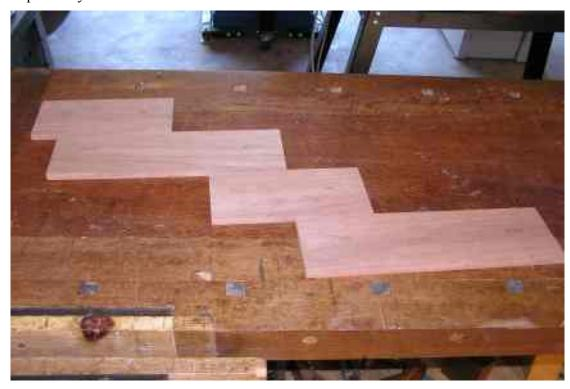
Lay the sides end to end in the order they will be assembled, and mark each pair of ends so that they can be assembled in the correct order.
