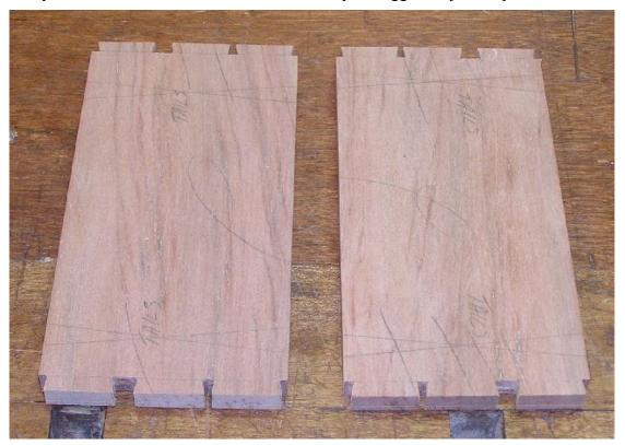
At this stage, if the box is to have floating panels or till supports, the slots should now be cut by router. This box is to have till supports.
