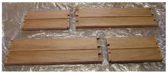
Select a glue that will give you sufficient time to glue up, while providing adequate strength. Epoxy will give lots of time, but is expensive and can be messy. PVA is a good option, as it allows reasonable time, can be accurately placed and is reasonably priced and strong. Aliphatic (yellow) glue has the same advantages, is stronger but sets more quickly. If you use it for dovetails, be prepared to work quickly. All these glues set more quickly on hot days.
