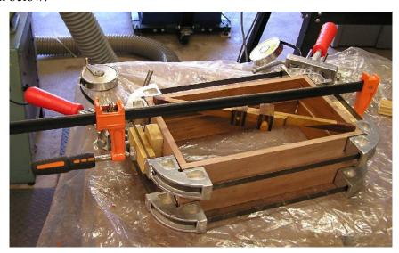
If the box is not square, place a clamp lengthwise along the box, at a slight angle. The clamp should be angled slightly in the direction of the long diagonal. This clamp does not need to be very tight. Check the diagonals frequently as the clamp is tightened.
