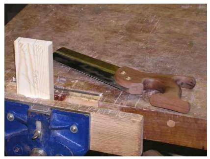
Remove the bulk of the waste between the pins. This can be chiselled out, or removed using a band saw or scroll saw. Whichever method you use, do not remove the waste all the way to the depth lines. Stop about 0.5 - 1 mm short.
