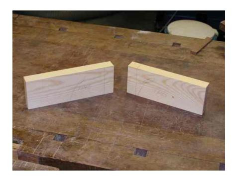
Using a dovetail gauge or bevel gauge, mark out the ends of the pins with a scriber. Darken the lines with a pencil and mark the waste that is to be cut away.
