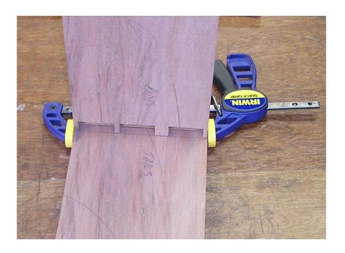
Using a try square and awl, mark the position of the tails on the ends, and extend them down to the pencil line on the outside.
