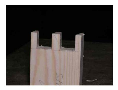
Use a bevel-edged chisel to pare down to the depth line. It helps to make a set of paring guides as shown below. Set the work piece in the vice with the depth lines level with the top of the paring guides. Rest the chisel on top of the guide, pointing slightly upwards, and pare away a thin sliver. Repeat this, gradually bringing the chisel towards level, but do not go through to the other side. You should be able to feel the blade of the chisel in the depth line when the cut is deep enough
