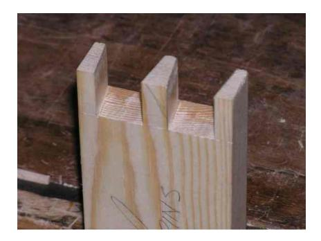
Sit the pins on the tail piece, making sure that the edges of each piece are in line. The inside face of the pin piece must sit exactly on the depth line of the tail piece. It may be convenient to either lightly clamp the pieces or have someone hold them while you mark the tails.
