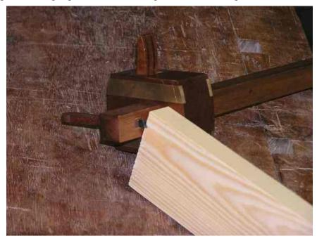
With the cutting gauge held against the ends of the timber, mark the depth of the tails and pins on the sides of the pin piece and all round the tail piece. There is no need to cut deeply. The score marks may be darkened with pencil to make them more visible.
