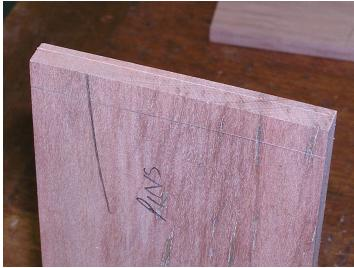
Using a scratch awl, mark the location of the pins on the scribed line. If the lid of a box is to be separated later, remember to allow a wide pin for the saw kerf. Then use a bevel gauge set to the desired angle, or a dovetail gauge, to et the pins out on the end of the piece. Use a try square to set out the pins on the inside face. Mark the
