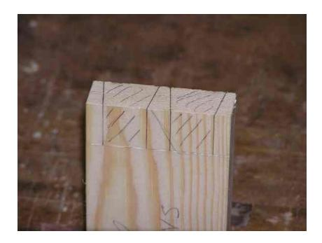
Using a dovetail saw, Japanese saw or fine tenon saw, cut along the waste side of the marked lines. Aim to have the saw bisect the line, but do not cut into the pin. If there is excess waste it can be removed later. Be careful to cut only as far as the depth lines on the inside and outside faces. It is better to not cut far enough than to cut too far.
