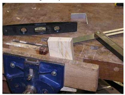
Remove the waste from between the tails, as you did with the pins. Again, do not remove it all the way to the depth lines.
