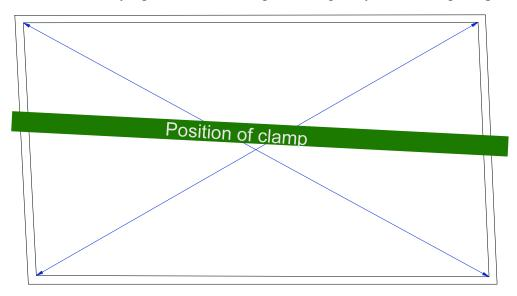
Leave the box clamped up long enough for the glue to set – several hours for PVA, up to 12 hours for epoxy. Remove the clamps, and carefully remove any squeeze-out using a sharp chisel. If you used epoxy glue, beware of sharp chips as the excess breaks away. These can cut skin or damage your eyes.
