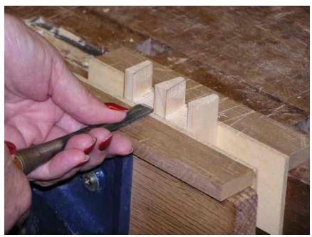
If necessary, tidy up the sides of the pins so that they are flat, square and accurate.
