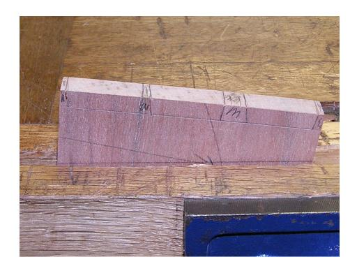
Cut along the marked lines. Aim to bisect the scribed line with the saw on the waste side of the line. Cut carefully to the marked lines on the inside and outside faces, but do not go past them. Cut out the bulk of the waste using a scroll saw, fret saw or chisel, but leave a little waste to be squared up accurately.
