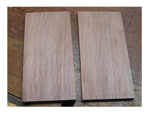
With the bevel gauge, mark lines at the angle of the dovetails, across the inside face, in both directions.
